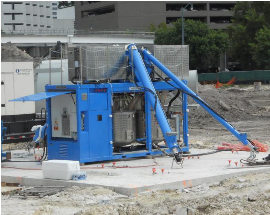
Mixing plant OM 1000/2-48 with hydraulically driven charging augers
