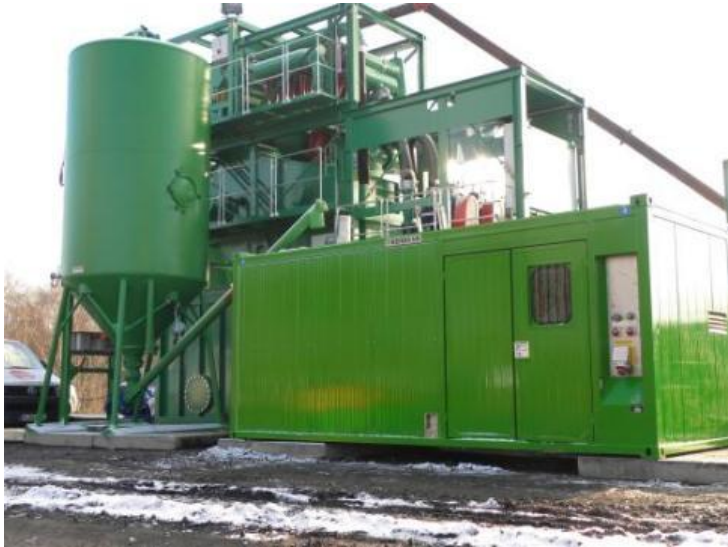
Mixing- and grouting container type MIC Application: Bentonite lubrication for pipe jacking
